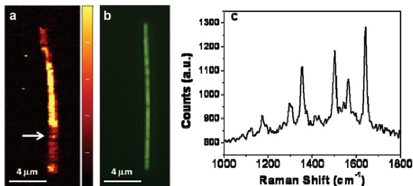
Figure 5. SERS of R6G adsorbed on the nanobuckles along silver nanowires: (a) confocal Raman mapping based on intensity of the R6G Raman peak at  $1650\text{ cm}^{-1}$ , (b) optical image of the same silver nanowires with buckles. (c) Raman spectrum of R6G corresponding to the location indicated by an arrow mark in the Raman mapping.
