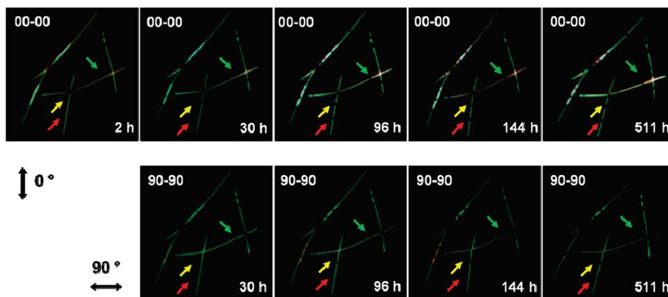
Figure 3. Optical reflection micrographs of the same silver nanowires captured at the different times. The images in the top row are captured at (0,0) configuration in polarization. The bottom row images are captured with a (90,90) configuration. Images are  $25 \times 25 \mu\text{m}^2$ .
