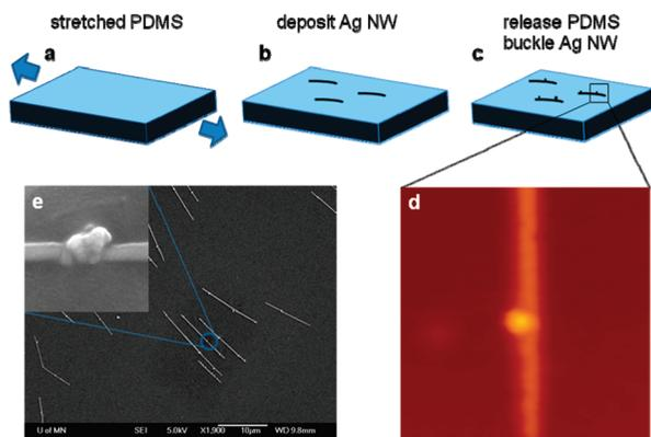
**Figure 1.** Schematics and images of silver nanobuckles: (a–c) compression-induced silver nanobuckles formation by depositing silver nanowires onto a prestrained PDMS substrate; (d) AFM image of silver nanobuckle formed on a silver nanowire (image size:  $5 \times 5 \mu\text{m}^2$ ); (e) SEM micrograph of silver nanobuckles along the silver nanowires. (Inset) A higher magnification ( $25000\times$ ), side-view (tilt angle,  $30^\circ$ ) SEM micrograph of a silver nanobuckle.
