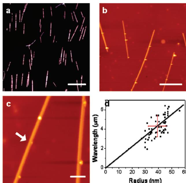
**Figure 2.** A graph of distance between silver nanobuckles with respect to silver nanowires diameter. (a) Optical reflection micrograph of silver nanobuckles along silver nanowires. Scale bar is 20  $\mu\text{m}$ . (b) AFM image of nanobuckle on silver nanowire. Scale bar is 5  $\mu\text{m}$ . (c) A higher resolution AFM image of silver nanobuckles. Scale bar is 1  $\mu\text{m}$ . (d) The dependence of distance between silver nanobuckles with the diameter of silver nanowires.
